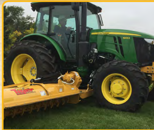
NEW DRAFT BEAMS WITH HIGHER GROUND CLERENCE
